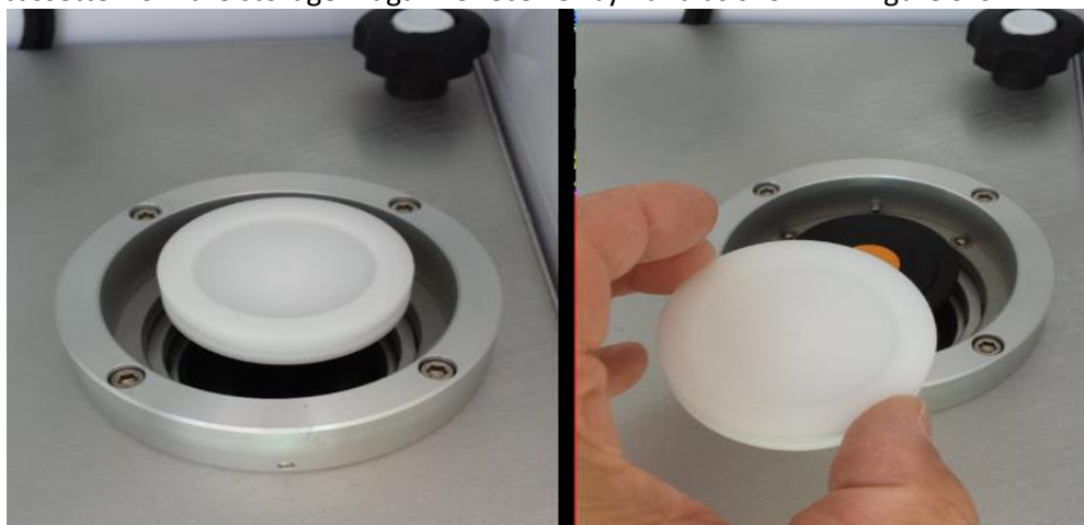
Figure 9-6 Removing the External Leak Test Cassette
