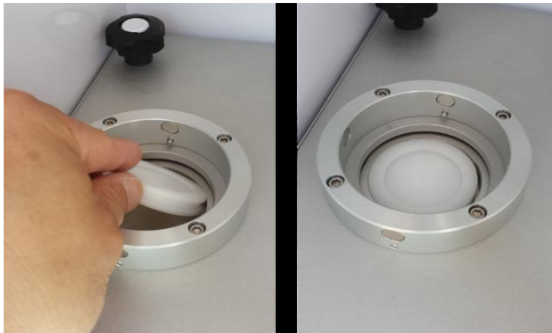
Figure 9-8 Inserting the Internal Leak Test Cassette
