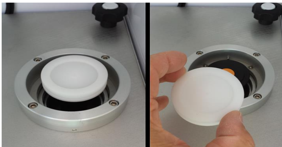
Figure 9-11 Removing the Internal Leak Test Cassette
